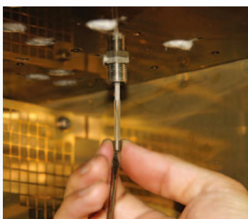
Simple nozzle replacement supports both capillary and packed columns.
