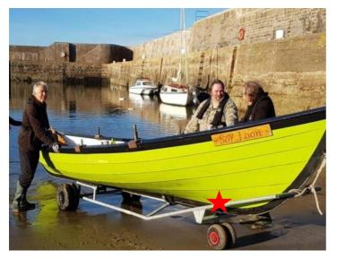
Launching Trolley: used to walk a boat to the launching spot; designed to be pushed into the water so the boat can be floated off and on easily. The \*front wheel swivels and should be aligned forward for going downhill. It is not suitable for transporting a boat on public highway.
