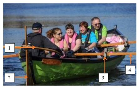
(rollocks), 4 U shaped wooden fixtures that sit over the tholepins to hold the **oars** in place.
