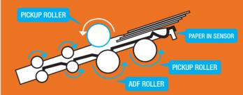
The Advanced Reverse Roller is a paper separation system for exceptional paper feed efficiency, helping to prevent loss of content and keep scan flow moving.
