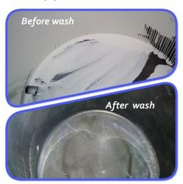
Basca supported the client to analyze facts and figures of the present situation, suggesting possible solutions to wash the containers in automatic way. Then a washing test at Basca facilities has been done to find the most suitable machine configuration. One the desired machine configuration has been finalized we have supplied a Basca Washing Machine equipped with a 200 bar pump to spray the water on the tank surface granting a perfect cleaning in about 5 to 8 min/tank.
