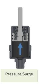
Water Hammer Arrester is a cylindrical-chamber with double sealing. The O-Ring divided the chamber into two areas. When installed on-line, spring in the Dry area being compressed by the line pressure. When Water Hammer occurs, the surge pressure & vibration are being absorbed by spring inside the Dry area.
