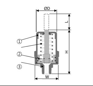
Applied liquid: Water Max. Working Pressure: 10 bar Installation Connector: PT Male Max. Working Temperature: 90 °C
