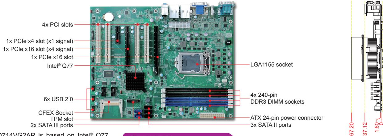
RUBY-D714VG2AR is based on Intel® Q77 chipset and desktop processor sku like Core™ i7 and i5. Built with flexible PCI express expansion and bifurcation feature, it can support two I/O interface cards and can also suitable for Medical, Industrial Automation, and Digital Signage applications.
