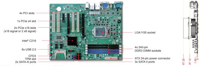
RUBY-D715VG2AR is based on Intel® C216 chipset and workstation sku like Core™ i3 and Xeon® E3-1200 series processors. Built with flexible PCI express expansion and bifurcation feature, it can support two I/O interface cards and can also suitable for Medical. Industrial Automation, and Digital Signage applications.
