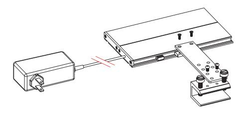
Attach Sump Arm Bracket to the Euro Brace Arm Module. Attach to Sump Neck Module
