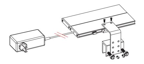
Attach Sump Arm Bracket to the Sump Arm Module. Attach to Sump Neck Module
