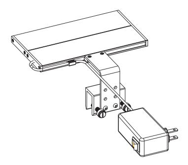
Thread plug's wire through the Cord Manager and place in sump.
