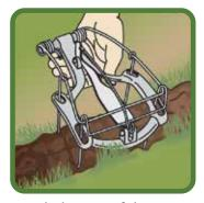
Mark the top of the run with the **Loops** of the trap.
