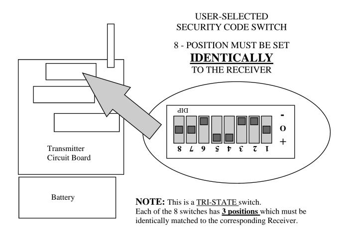
These code switches are fully compatible with 8-position Two-State On/Off switches by using the "+" setting as ON and the "O" setting as OFF.
