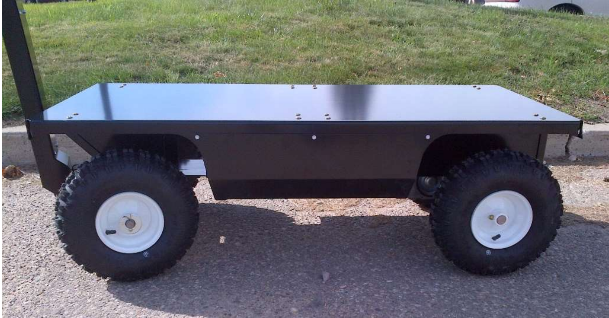
Figure 5: Single Motor, Single Battery, 1000lbs payload
