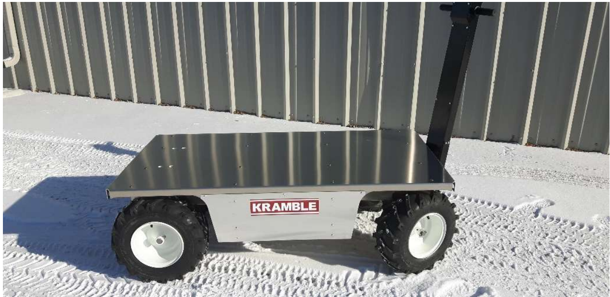
Figure 7: Heavy Duty Cart – Dual Motor, 4 Battery, 4000lbs Payload
