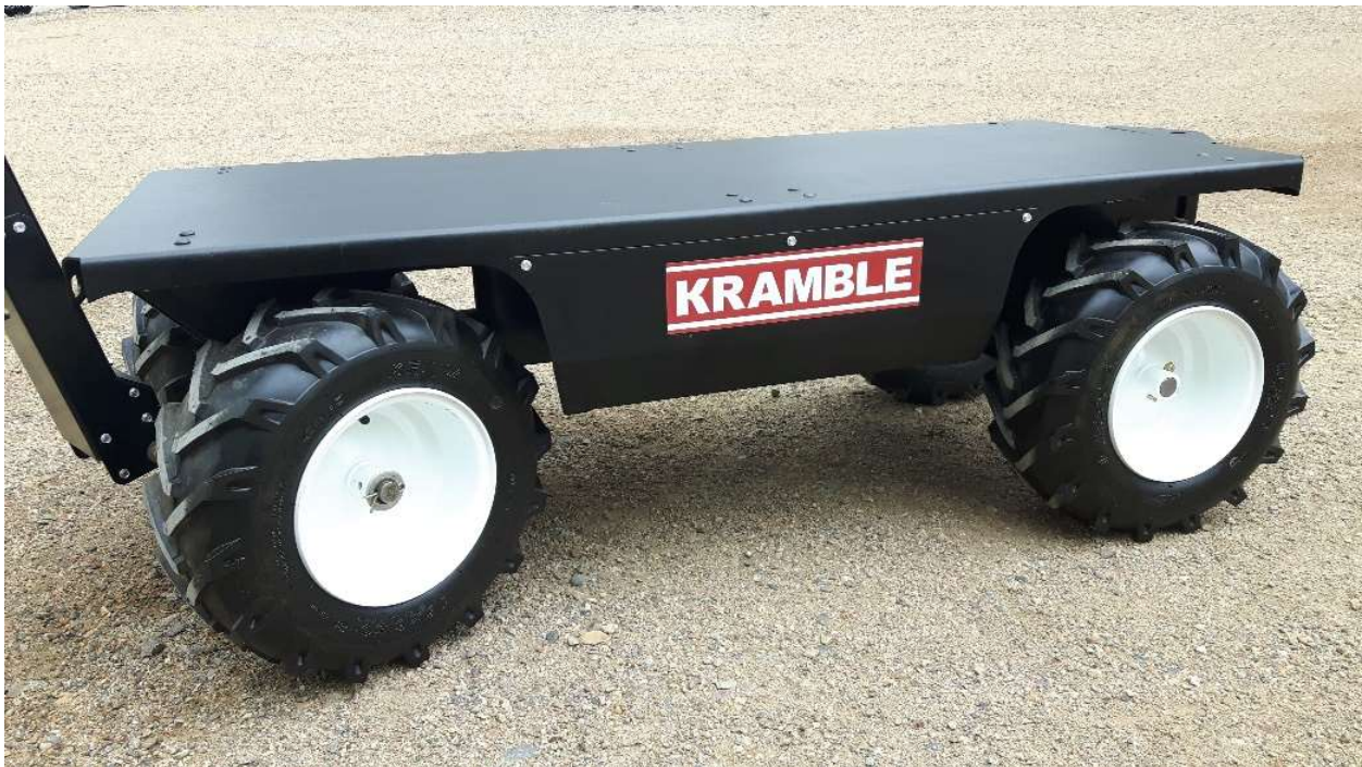
Figure 6: Single Motor Single Battery 2500lbs Payload
