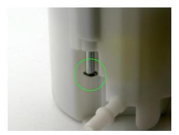
2 – to remove the center section of the assembly from the bucket, there are 2 spring tabs and 1 clip. While pulling on the center section of the assembly, lift the middle tab (black circle) and squeeze the outside tabs together (green circles). Once all 3 tabs and clip are loosened, separate the center assembly from the bucket
