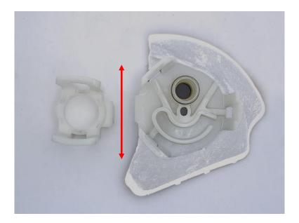
5 (2010-2012) – transfer the outlet spacer from the OE pump to the DW pump and install 1 of the new o-rings from the installation kit. Install the new, clipped pre-filter on the DW300c and install into the center assembly while connecting the electrical connector and snapping the pump retainer in place
