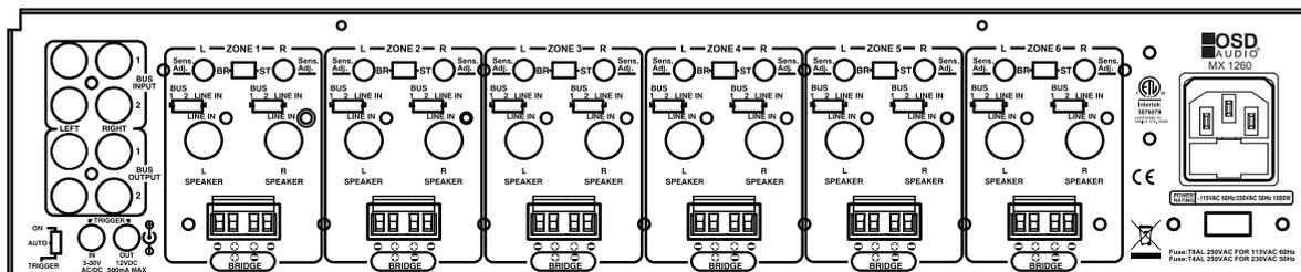
Connect the right or left output from the audio source to the right or left input of the zone you are bridging. Repeat this for each zone you want in bridged mode.
