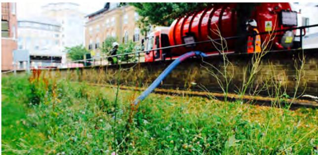
Trialling a SDS feature in a 'simulated flooding event' (credit: Groundwork).
