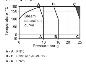
The product **must not** be used in this region or beyond the body design conditions quoted in the table below as damage to the internals will occur.
