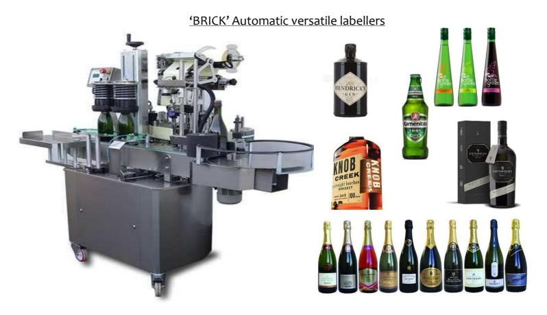
Compact, versatile machines for precise application of multiple labels onto round containers such as 'Champagne' bottles which may be tapered or shaped, Also square bottles, ovals, rectangular and other shapes.
