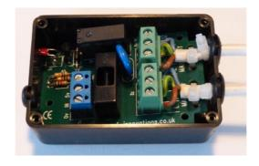
2. Once the product is assembled and shown to be working correctly, we recommend using hot melt glue where the cable enters the screw terminals to prevent strands of wires accidentally touching each other.
