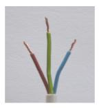
Cable ties should be used to provide strain relief and prevent the mains cable pulling out of the screw terminal. One should not just depend on the screw terminals to anchor the cable. The cable must move less than 2mm for a force of 30N (i.e. the weight of 3 x 1kg bags of sugar).
