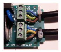
Once the product is assembled and shown to be working correctly, we recommend using hot melt glue where the cable enters the screw terminals to prevent strands of wires accidentally touching each other.
