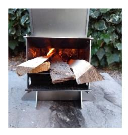
Load the upper part of the firebox with some kindling. One method of lighting is to use some crumpled up newspaper and light this first which in turn should get the kindling lit. (a few drops of cooking oil on the paper will help this process). Then add bigger pieces of wood till the fire gets going. The lower part of the firebox is the air intake and must not be blocked.
