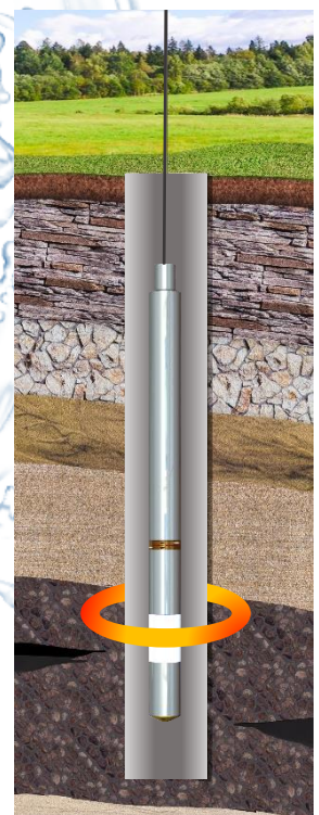
BMR tool interrogating surrounding rock (orange ring)
