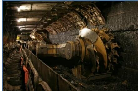
Predicting under what conditions coal walls may pose outburst risk requires knowledge of coal gas content and coal cleat permeability, as these parameters dictate how much and how fast free gas can accumulate behind the wall. That information enables mine operators and regulatory agencies to identify the threshold gas content below which mining is deemed safe. Knowledge of gas content and permeability also enables mine operators to:
