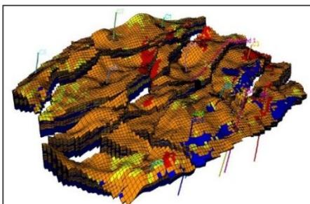
Furthermore, coal seam properties can vary significantly, over very short distances, both laterally and vertically. As such, successful gas management plans require access to realistic distribution maps of gas content and permeability, based on closely spaced, accurate measurements to adequately capture this heterogeneity.
