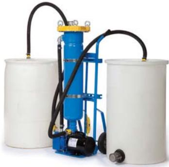
The FloWash Basic Filter Cart is an easy-to-deploy mobile system that helps keep your shop floor fluids cleaner for improved production efficiency. It can be used on-line or as a stand-alone filter station. Save on replacement fluids as well as the associated disposal costs.
