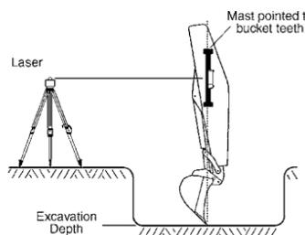
1. Position the machine and dig to the desired finished elevation.
