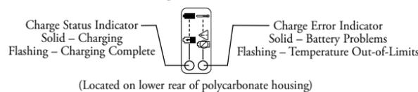
**Charge Status Indicator:** The LED remains solid when the batteries are charging. The LED flashes when the batteries are fully charged. When the batteries are charged, unplug the charger from the outlet, and remove the cannon adapter from the accessory connector.
