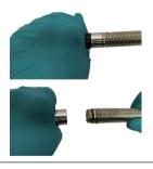
Continue to unscrew the spring by turning it in the counter-clockwise direction.
