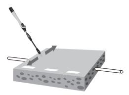
Sweep the locator left to right along the suspected route of the cable. As the locator approaches the cable the meter reading will increase. Pinpoint the position by detecting the largest signal.
