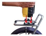
2. Lower the control module into the mounting blocks.
