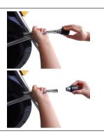
**Installing:** Remove any excess dirt that might come into contact with the gold pins or green circuit board. Check that the O-ring is in good condition.
