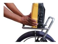
Push the control module backward until locked into place.
