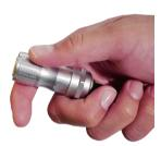
b. Line up the red dot on the interconnect cable plug with the red dot on the control module's socket. Insert the plug into the socket and release the knurled ring.
