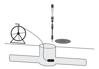
Hold the locator above the Sonde at ground level. Adjust the sensitivity of the locator by pressing the "+" or "-" pushbuttons to keep the signal on scale. Rotate the receiver until the maximum signal is detected.
