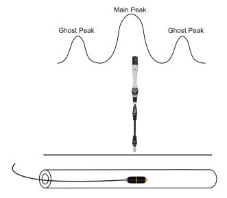
Now push the Sonde a few feet into the pipe. Stop and re-locate the Sonde. The direction of the Sonde can be confirmed by holding the locator vertically and rotating it on its axis until the largest signal is detected. The Sonde will then be pointing at right angles to the display.
