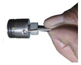
4. Pull the floating camera nut up and over the lanyards.
