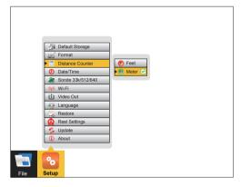
6. Press the ESC key to return to the main Setup menu, press ESC twice to return to the main screen.
