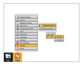
Use the **up** ♠ and **down** ♣ arrow keys to highlight and select the .bin or .soc file and press **Enter**.
