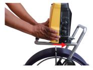
Unspool enough of the interconnect cable from the reel to allow its plug to reach the socket on the control module. Be aware of any excess cable around the cable cage that may become tangled when the cage starts spinning. Use the Velcro strap attached to the interconnect cable to secure the cable in place.
