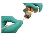
3. Feed the two lanyards through the floating camera nut and insert into the lanyard slots. Make sure that the lanyards are straight and not tangled in the coiled cable.
