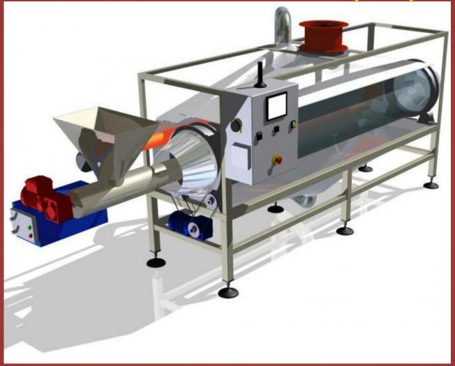
The drying process takes place during the movement of material in a perforated rotating drum and is conducted by infrared and convection heating.
