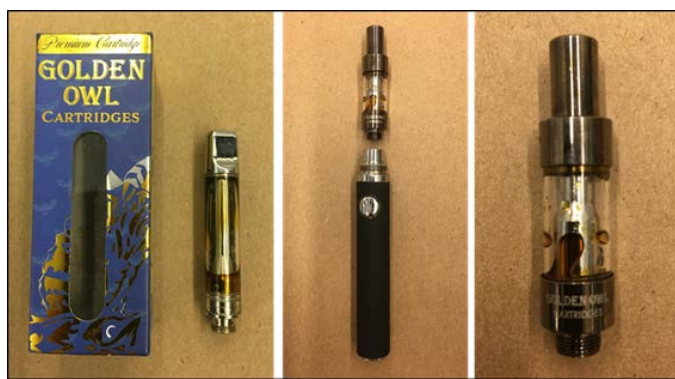
THC vape cartridge with packaging (Left). Positioning of how cartridge assembles to base (Middle). Close view of cartridge containing residue THC oil (Right). (Source: DC Department of Forensic Sciences)
