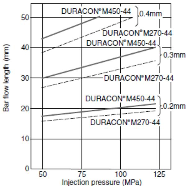
Fig. 2-6 Flowability in case of thin wall
