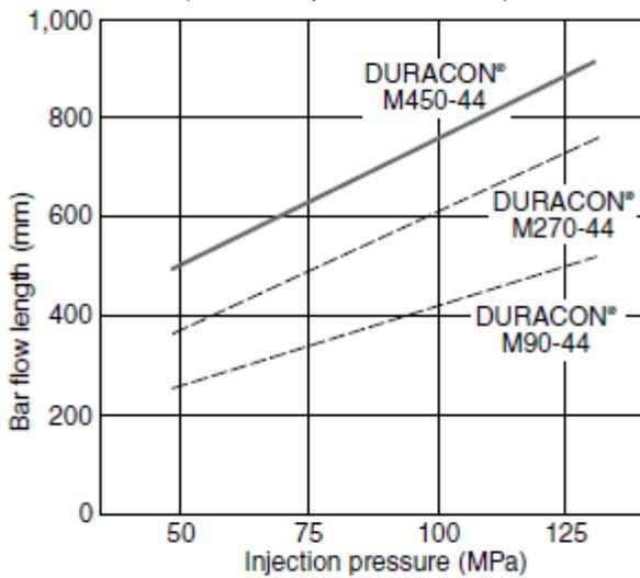
Fig. 2-4 Flowability at 2 mm wall thickness
