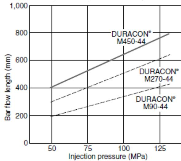
Fig. 2-5 Flowability in case of thin wall
