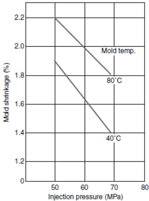
**Fig. 2-11 DURACON® M450-44 mold shrinkage ratio (3mmt)**
