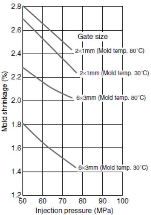
**Table 2-4 DURACON® M450-44 mold shrinkage ratio**
