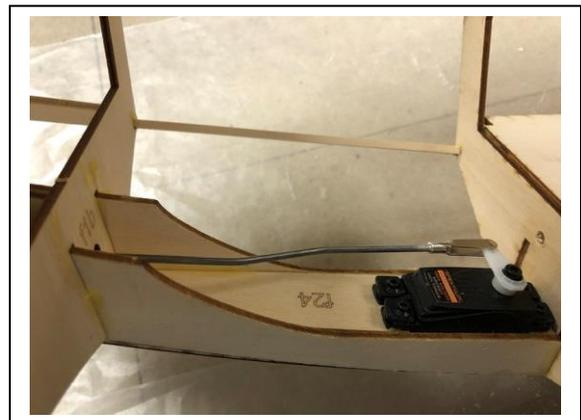
parts fit between the nylon block and the f22 keel parts. Sand them as needed for best fit.
