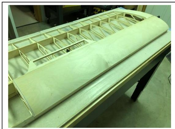
unique for both top & bottom and left & right. Each is labelled accordingly. The top sheeting requires all the tapered 48" long 1/32" skin plus a smaller section to reach the tip.
