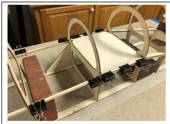
F26 is added to the top of the stringers between formers f6 and f7. Note the binder clips. We also like to use landscape paving bricks to help hold things in place.
