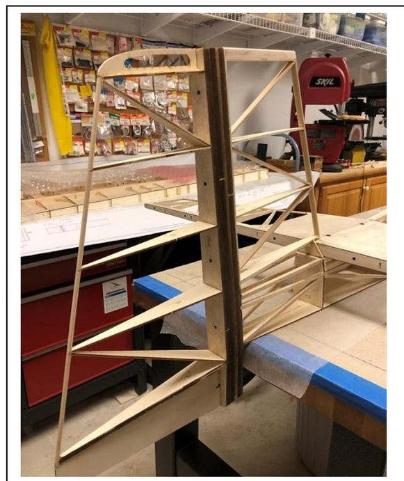
With the fuselage flat on the work surface and the fin plumb, set the stab on the fuselage and check alignment. When satisfied, drill a 1/16" pilot hole. Remove stab and check location of the pilot hole in f19. If satisfied, place the stab back on the fuselage and hold in place with a piece of 1/16" music wire or drill bit. Check alignment again and when satisfied, drill a second pilot hold as per the plan location.
