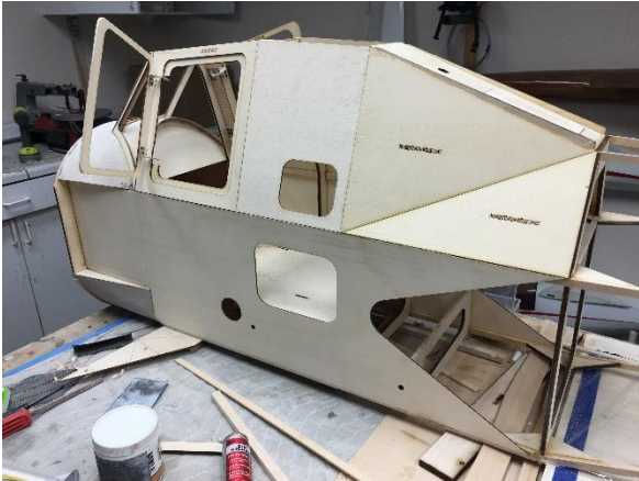
Front deck and lower fairings are sheeted with 1/64" ply.
