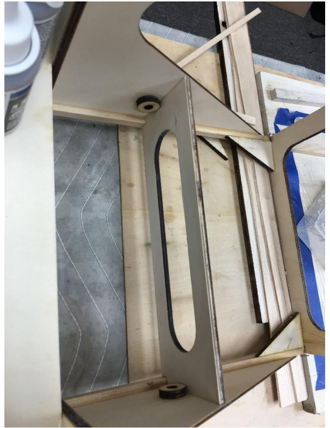
Now to build the Rear of the fuselage. This is done with the fuse positioned upright on the bench. Use a right angle devise to ensure the rear of the fuse at 90deg to the bench.
