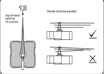
When you have finished the alignment, Install\* the battery (AA type) and adjust the time using the adjusting wheel at the back of the clock mechanism.
