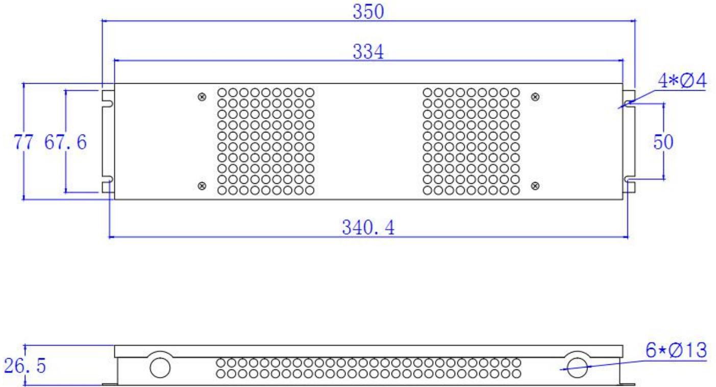
■ Real picture & Mechanical Specification of 50W Phase/Triac Dimmable Driver with junction box -2
