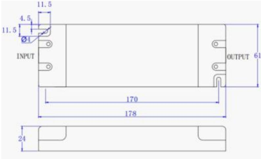
■ Real picture & Mechanical Specification of 50W Phase/Triac Dimmable Driver with junction box -1
