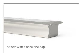
Designed for mudding in to drywall, Ankr 4 features flanges that make for a seamless installation. A countersunk hole is predrilled in the bottom of the channel every 4 inches for screwing into studs, making installation flexible and easy.
