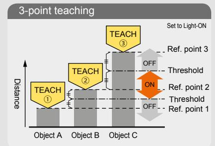
This is the method to set the threshold range by conducting the teaching at 3 points (detecting object A, B and C). After teaching, the reference points are automatically sorted in ascending order (reference point 1, 2 and 3). The thresholds are set at the midpoints between reference point 1 and 2, and 2 and 3, respectively. This is useful for detecting objects at different distances.
