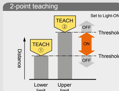
Press the button TEACH once for the lower (first point) and once for the upper limit (second point). This is useful for detecting objects at different distances.
