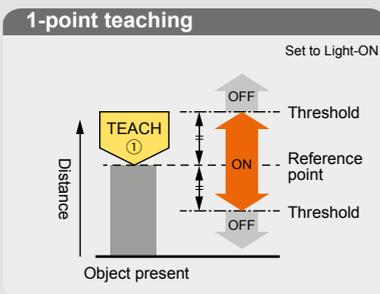
Perform 1-point teaching and the threshold range is set for the distance from the reference surface of the object to be detected.
