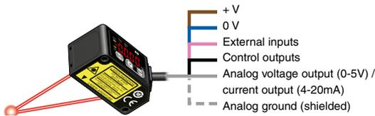
The sensor not only indicates measured values in mm, but also outputs analog voltage / current. The data can be used for various calculations and storage (logging) when the output is sent to a PLC + analog unit.
