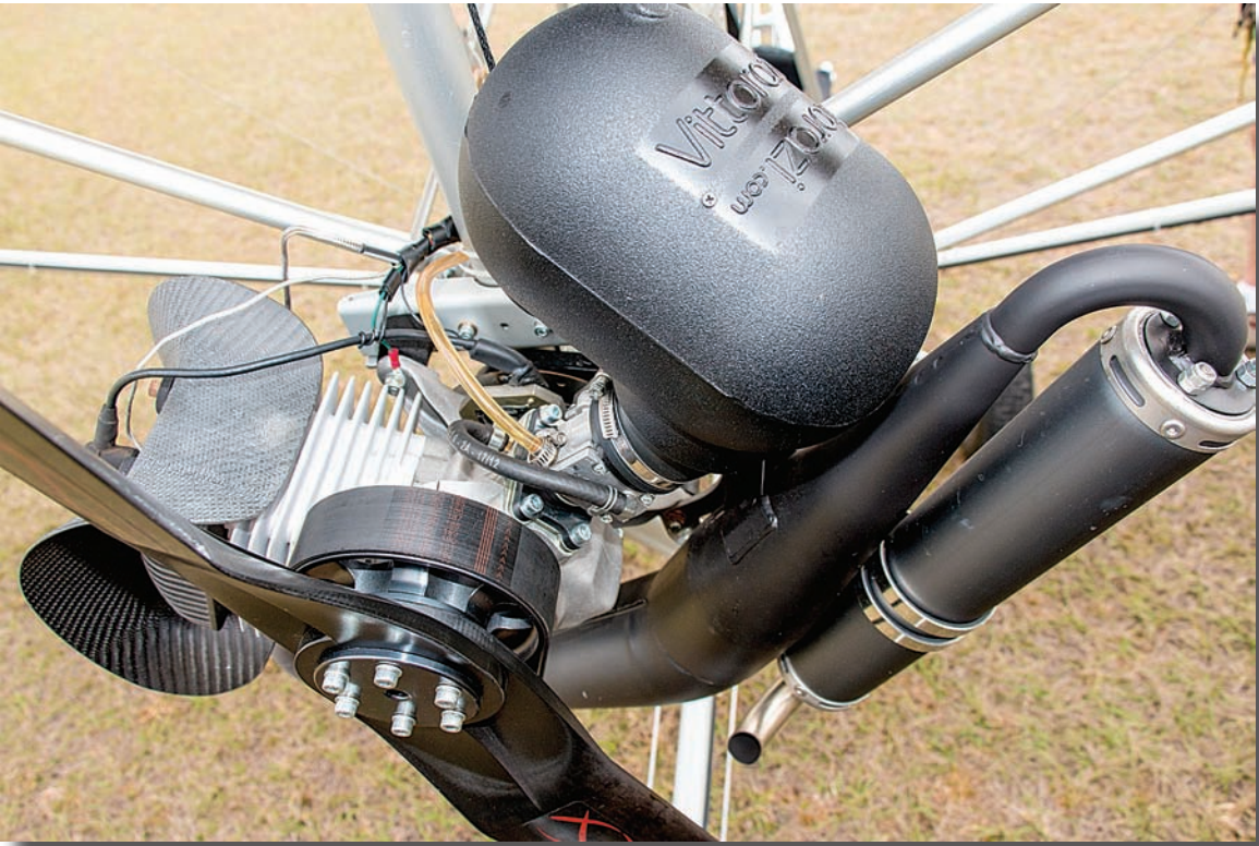
Above: The pneumatic Commelli recovery parachute is included in the kit price and empty weight of the Zigolo MG12. Upgrade to a BRS unit is an available option. Below: The Vitorazzi Master 185 powerplant. It's 25 horsepower, belt driven and free-air cooled. —PHOTO BY JAMES LAWRENCE
