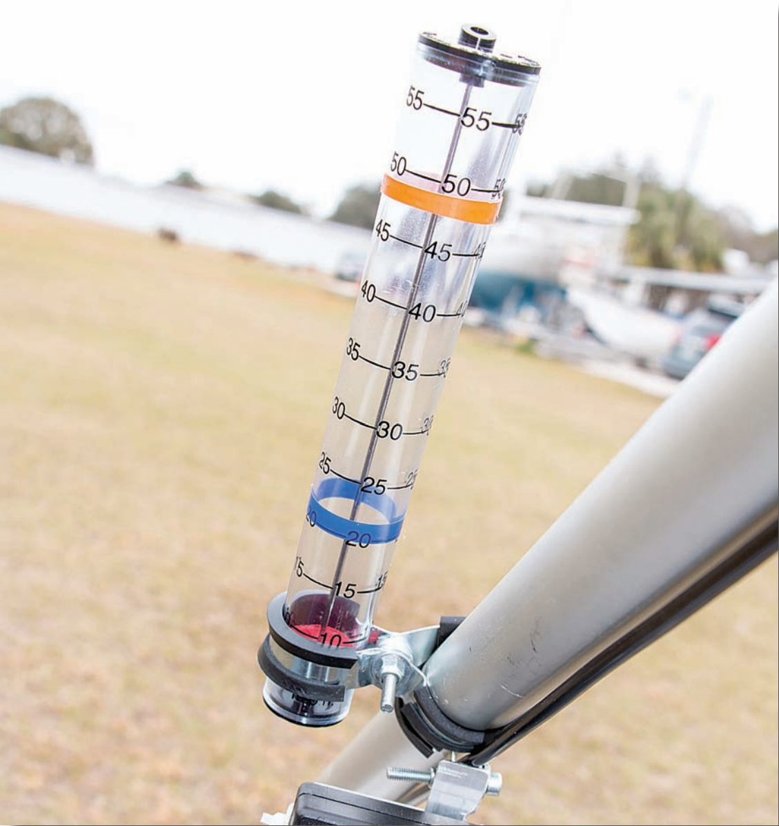
Above: A sparse cockpit array in ultralight tradition, putting the air in airplane. Below: the Hall airspeed indicator maps the MG12's typically motorfloater speed range.
