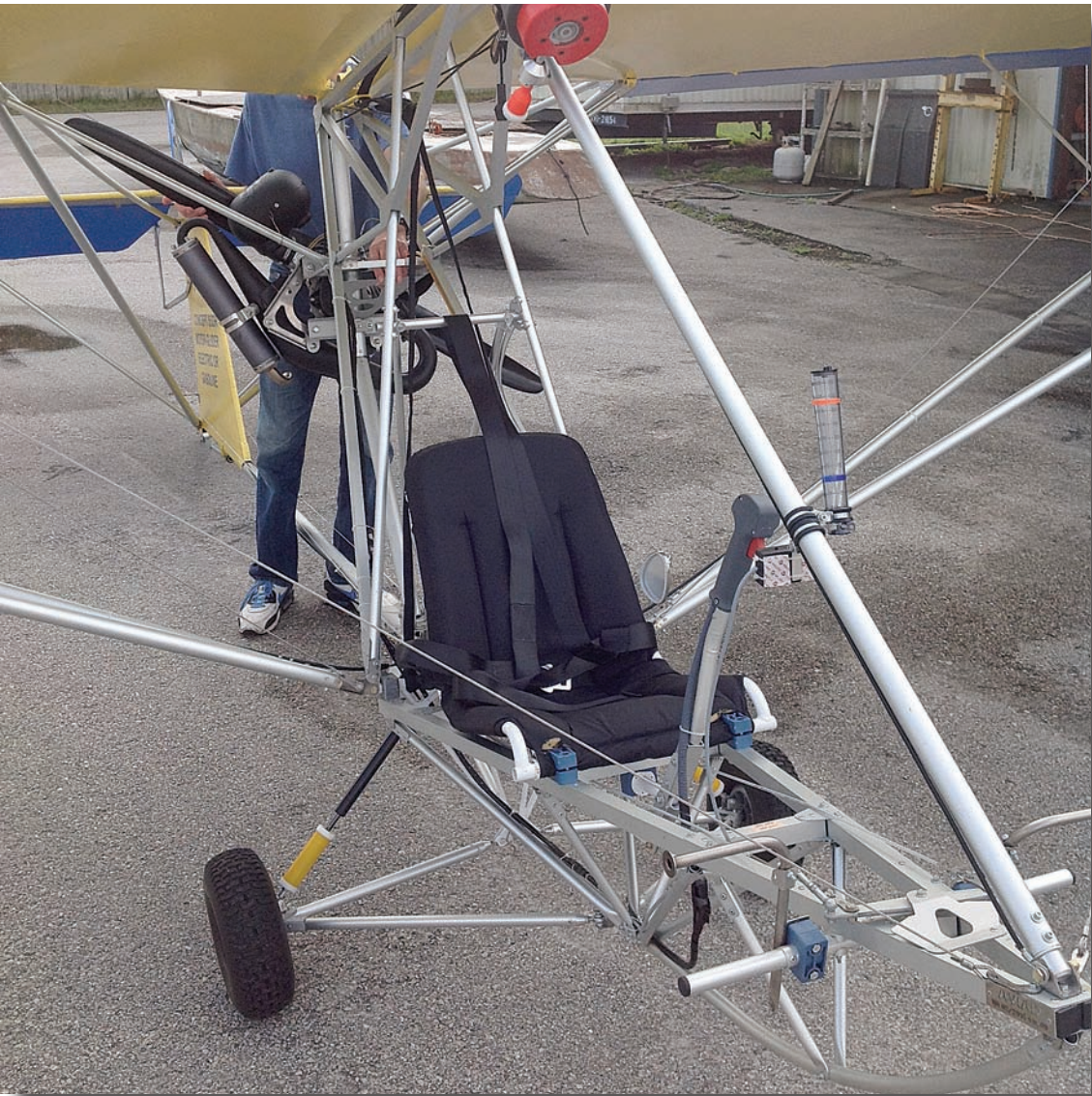
Above: A sparse cockpit array in ultralight tradition, putting the air in airplane. Below: the Hall airspeed indicator maps the MG12's typically motorfloater speed range.
