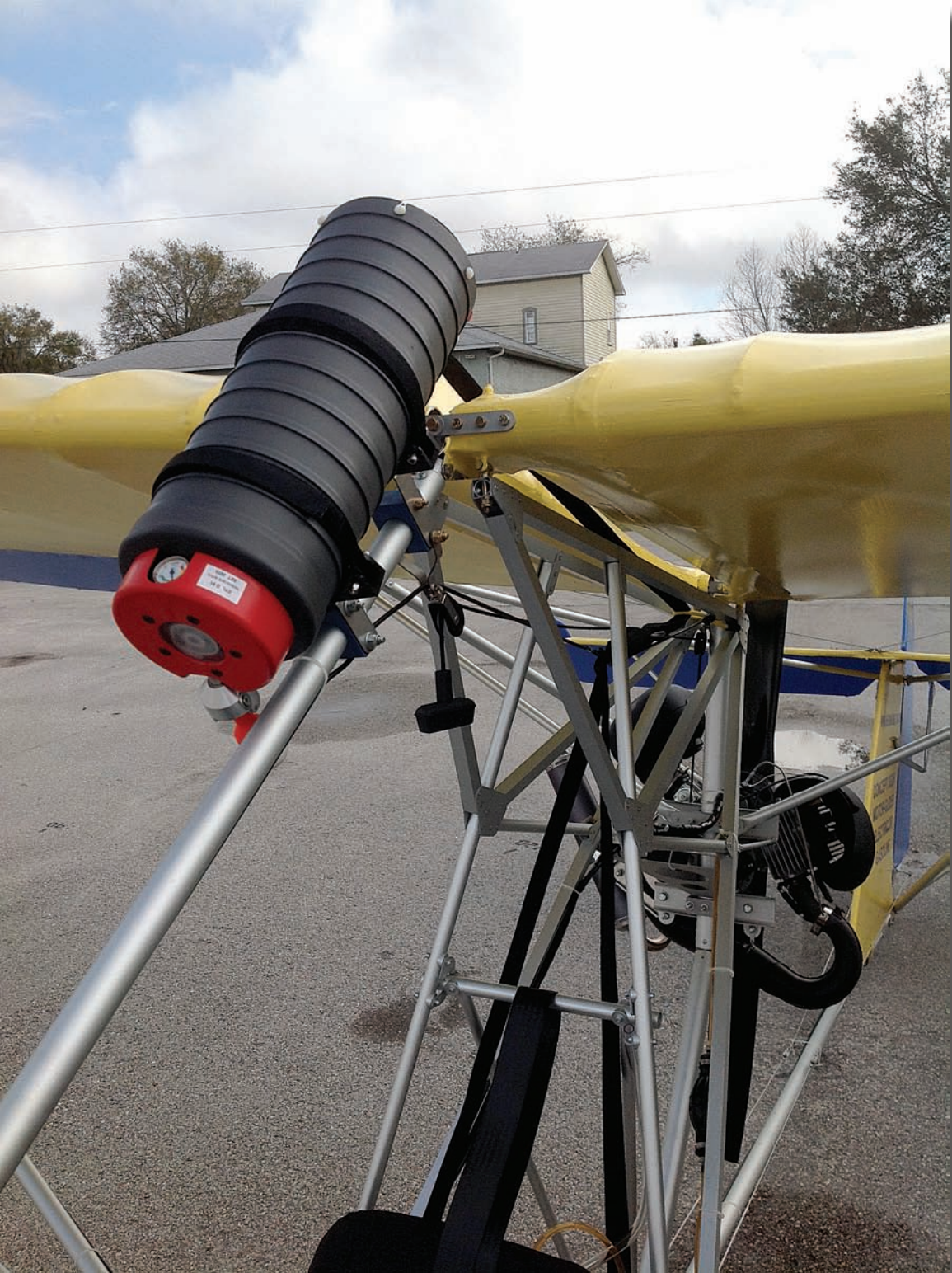
Above: The pneumatic Commelli recovery parachute is included in the kit price and empty weight of the Zigolo MG12. Upgrade to a BRS unit is an available option. Below: The Vitorazzi Master 185 powerplant. It's 25 horsepower, belt driven and free-air cooled. —PHOTO BY JAMES LAWRENCE
