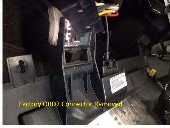
3. Insert the new OBD2 connector from security module bypass into the trucks OBD2 bracket.
