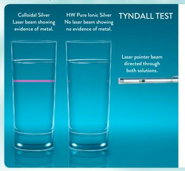
Normally when a laser is shone through a liquid other than distilled water, a path of light can be seen similar to when you shine a torch through smoke or fog.
