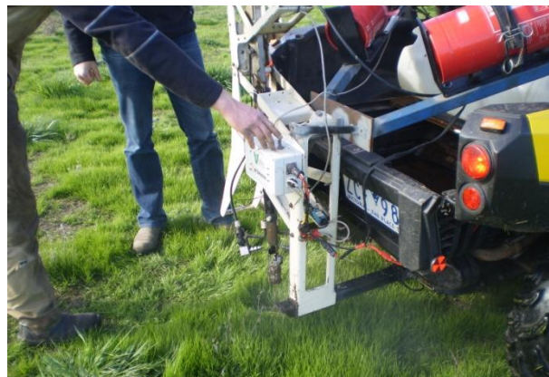
Figures 3 & 4; Precision Agriculture pH testing rig
