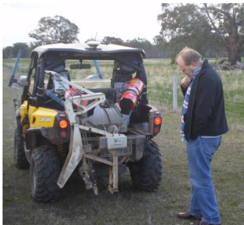
Figures 3 & 4; Precision Agriculture pH testing rig
