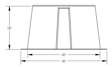
NOTE: Includes (4) 3/8x1.5 SST Hex Bolts, (4) 3/8 SST Hex Nuts, (8) 3/8 SST Flat Washers, (4) 1/2 SST Flat Washers
