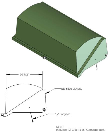
Includes (2) 3/8x1.5 SST Carriage Bolts, (4) 3/8 SST Flat Washers, (2) 3/8 SST Lock Nuts, (2) 3/8x1/2x5/8 SST Spacers
