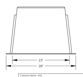
NOTE: Includes (4) 3/8x1.5 SST Hex Bolts, (4) 3/8 SST Hex Nuts, (8) 3/8 SST Flat Washers, (4) 1/2 SST Flat Washers
