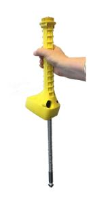
With your other hand, screw on the plate, making sure that the smooth side of the plate is uppermost (ribbed side closest to the meter).
