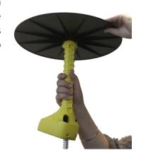
3 Turn the plate meter the correct way up (plate down) and place it on the ground. The grooved rod will protrude out of the shaft. With one hand hold the grooved rod and with the other hand, screw on the black plastic handle. Be careful not to displace the small rubber Oring on the top of the rod.
