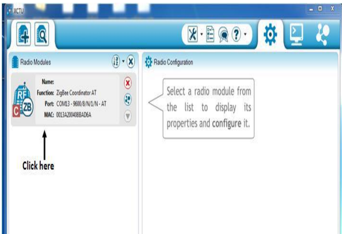
Fig 22: Selecting coordinator for configurations
