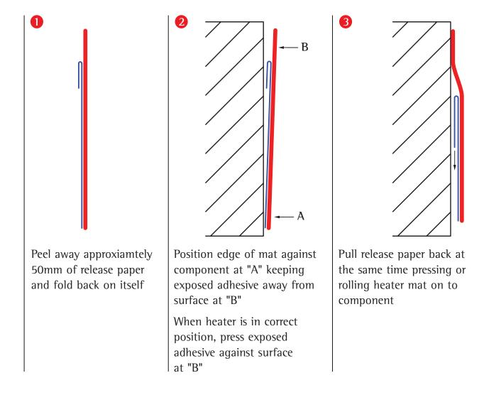
Note. Once heater mat is installed it cannot be re-applied
