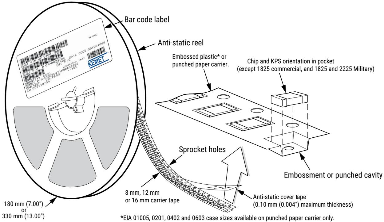
**Table 4 – Carrier Tape Configuration, Embossed Plastic (mm)**
