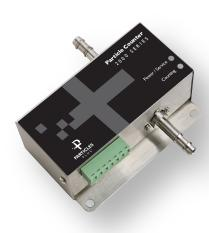
The Particles Plus 2510-1 Remote Particle Counter measures 0.5  $\mu$ m and 5.0  $\mu$ m with a flow rate of 1.0 CFM (28.3 LPM). Integration is easy into a real-time monitoring or building management system via Modbus <sup>TM</sup> RTU or ASCII. The P231 is the smallest remote particle counter in the market and has easy mounting options. The Particles Plus 2510-1 complies with ISO 21501-4 and includes a 2 year limited warranty
