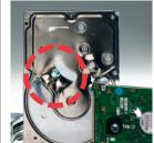
Punching a hole through the drive damages it irreparably, rendering it unreadable.
