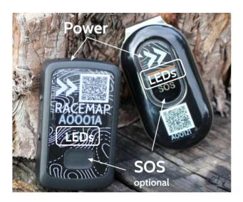
**LED Signal Pro GPS Tracker** Standard GPS Tracker network searching no LED Green continuously network reception Green every 2 sec en every 2 sec GPS searching Blue continuously **Blue** continuously GPS fix Blue off Blue every 2 sec charging Red every 1 sec Red continuously battery fully charged Red continuously no LED
