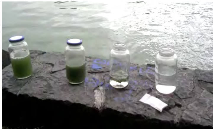
Biopolymer binds to algae protein, floats it to the surface for easy removal
