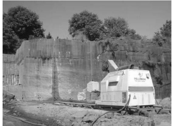
*The Wire Saw in action, note water mark on rock face marking the cut.*
