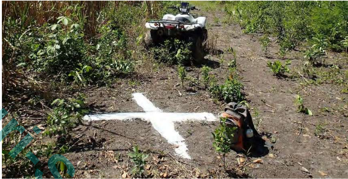
Figure 7: Placement of the GCP's with Lime and plastic
