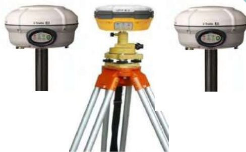
Figure 8: Trimble R4 smart base station and rover
