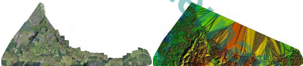
Figure 1: Orthomosaic and the corresponding sparse Digital Surface Model (DSM) before densification.
